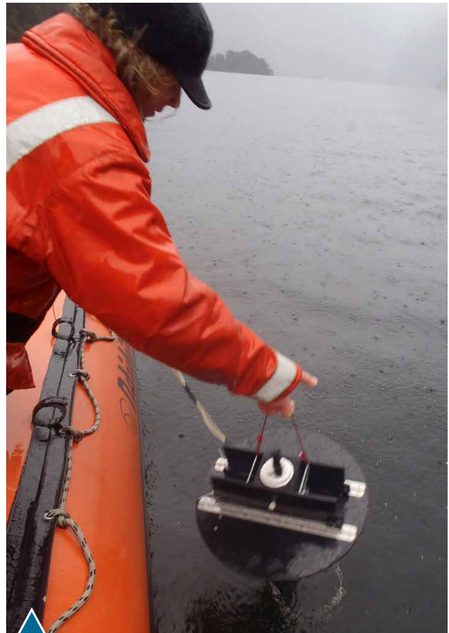
Joe O’Callaghan deploying SCAMP (Self-Contained Autonomous Micro-Profiler) through the very thin buoyant surface water in Doubtful Sound, Fiordland, New Zealand. While the rain may look unpleasant, it did a great job of keeping the sand flies away! Photo credit: Craig Stevens
