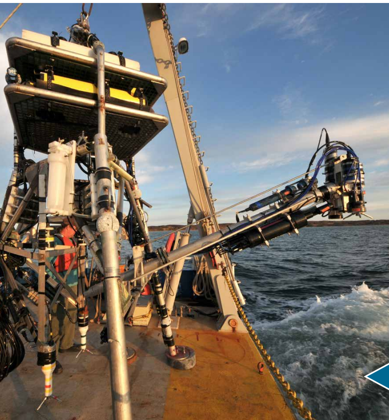
Aboard R/V Connecticut in October 2011 with a bottom tripod whose moving arm continuously profiles suspended sediment events at the seabed using acoustics, optics, and other methods simultaneously. Photo credit: Dann Blackwood, USGS
